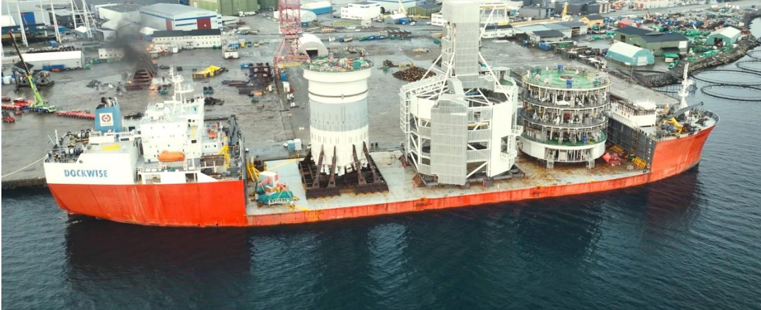
Johan Castberg: Turret, ready for Installation
